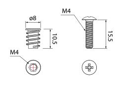
FORO BUSSOLA  $\emptyset6 \times 12.0$  built-in fitting  $\emptyset6 \times 12.0$
